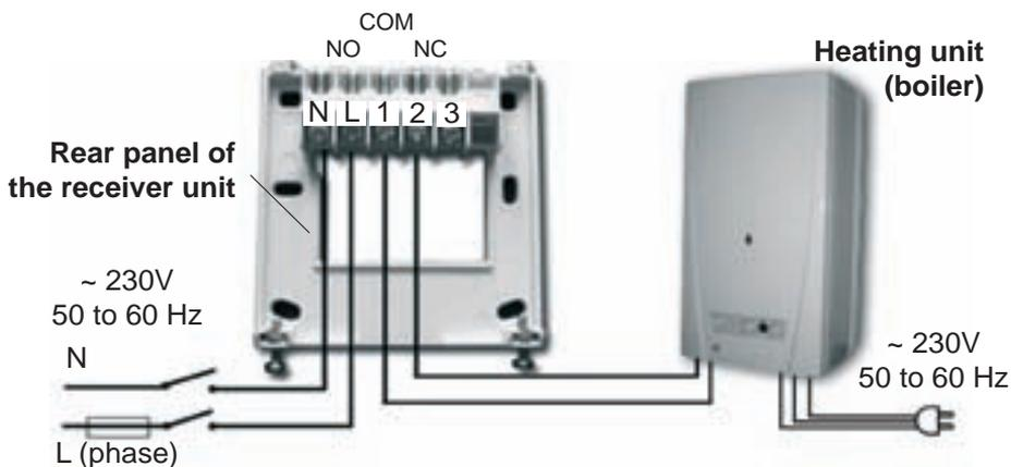
230 V mains voltage should be supplied to the receiver unit. We recommend using a fixed cable instead of a fork type connection for mains connection to avoid any unintentional de-energization of the device. We propose to connect the neutral wire of the network to point **N**, while the phase conductor to point **L**. We propose to interpose a switch so that the receiver unit can be de-energized if required.
