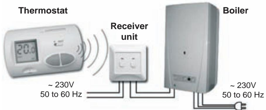
To increase the lifetime of the batteries, the thermostat will not transmit signals continuously. It will only send signals to the receiver whenever it should perform a switch.
